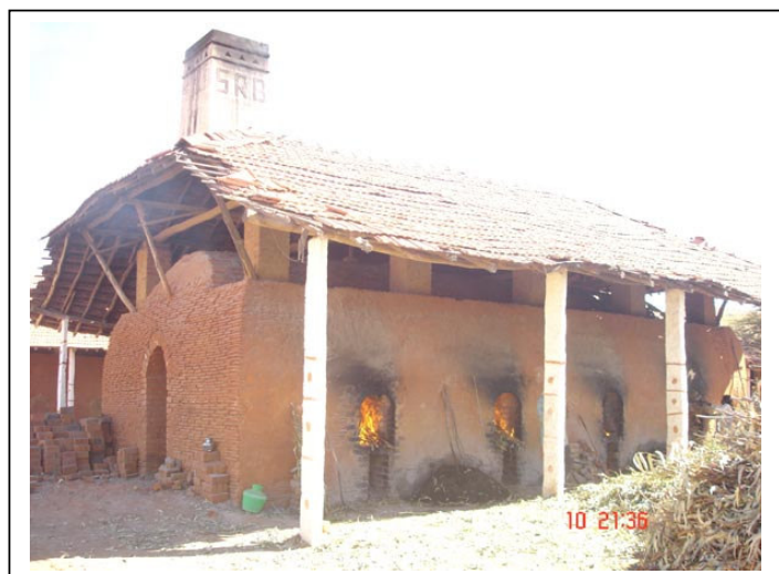
Figure 2 A view of downdraught kiln
