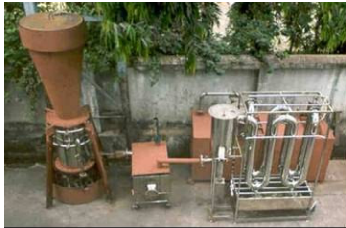
Gasifier system assembled for trial testing at Mumbai
